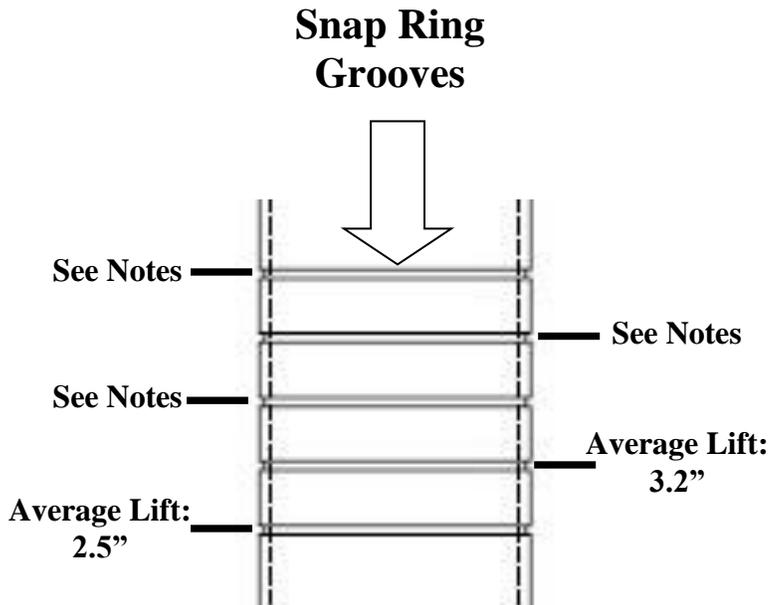
**Important:** Ensure that the snap ring is fully seated in the snap ring groove (you should be able to rotate the snap ring manually/by hand). **Note: Improper installation will cause permanent damage to the shock. Please refer to the Pro Truck Sport Damper instructions for more info regarding proper installation and fitment.**
