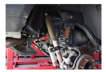
Reservoir should be mounted towards the bottom and pointing away from the axle on both side of the vehicle.
