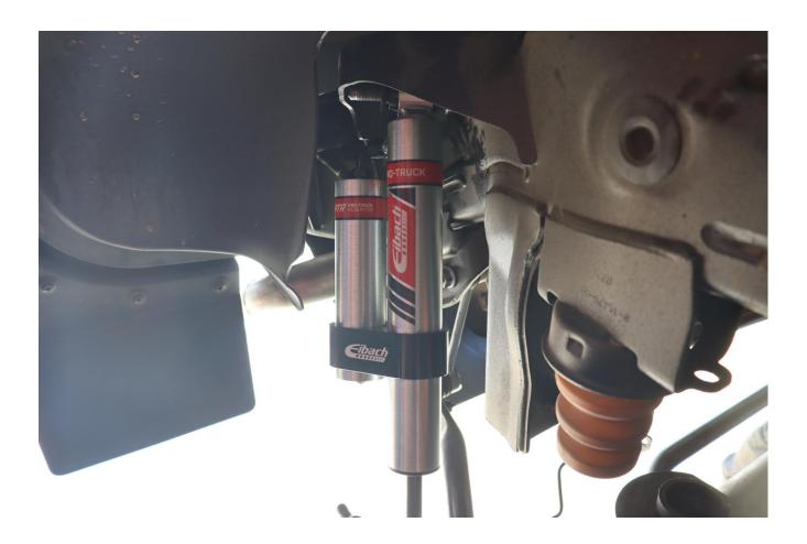
Reservoir should be mounted towards the top and pointing away from the frame on both side of the vehicle.
