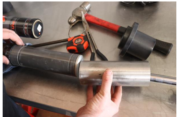
Remove the slider sleeve and crossover rings.
