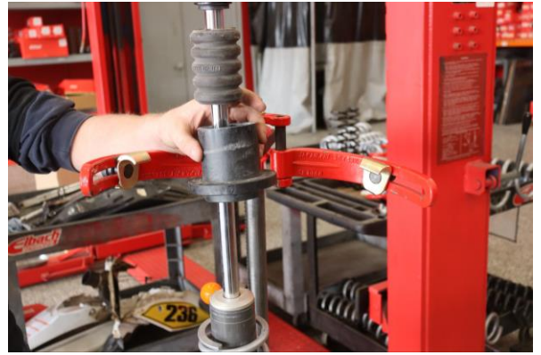
Remove OE spring slider.
