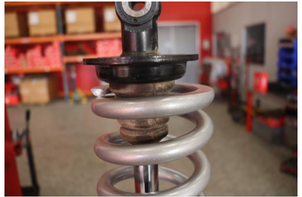
Compress the spring assembly and re-install the spring retainer.
