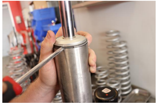
Remove the clip at the end of the shock body securing the slider sleeve.
